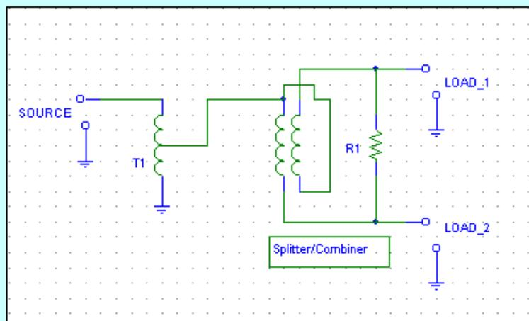
T1 is a 7-turn transformer tapped at 5 turns (1.4:1 turns ratio, 2:1 impedance ratio) step-down transformer. 73 material binocular cores are ideal for 100kHz to 30MHz applications.
