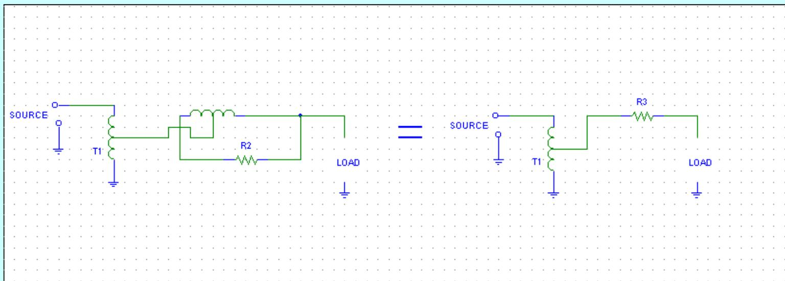
In a properly designed magic-T, R2 is twice the value of any port. This resistor is stepped down by the impedance ratio of 4:1 in the center tapped winding (no part designator) when a load port is opened. In a 50-ohm system, this effectively results in 25 ohms (R3) in series with the load impedance of 50 ohms. The resulting impedance of 75 ohms is doubled by T1 to 150 ohms. Assuming ideal components the input SWR, when the output is open on one port, is 3:1.
