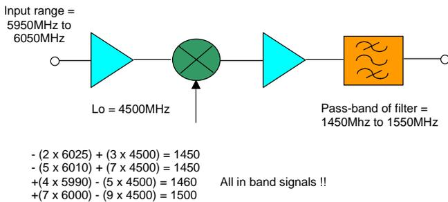
Figure 24 Example showing how intermodulation products in a down converter system can mix to produce products that fall within the pass-band and hence cannot be removed.
