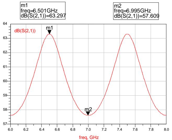
**Figure 5** Resulting gain plot from the ADS S-parameter simulation shown in **Figure 4**, showing the
