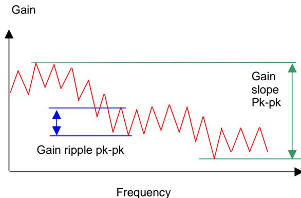
**Figure 1** Definition of gain ripple and gain slope where gain ripple is measurable, normally gain slope and gain ripple are used interchangeably.
