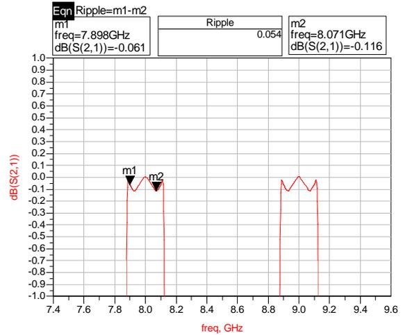
**Figure 15** Simulation result of the multi-path ADS schematic of Figure 14, verifying a gain ripple of ~0.055pk-pk.
