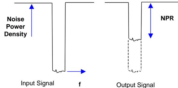
**Figure 17** Illustration of the *Noise Power Ratio* test, sometimes used to establish a more "traffic realistic" performance evaluation, resulting in the measurement of non-linearity (**NPR**).
