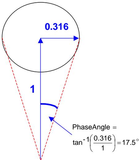
**Figure 3** Resulting signal phasor due to the introduction of the feedback loop gain phasor of magnitude -10dB (which equates to a power of 0.316)
