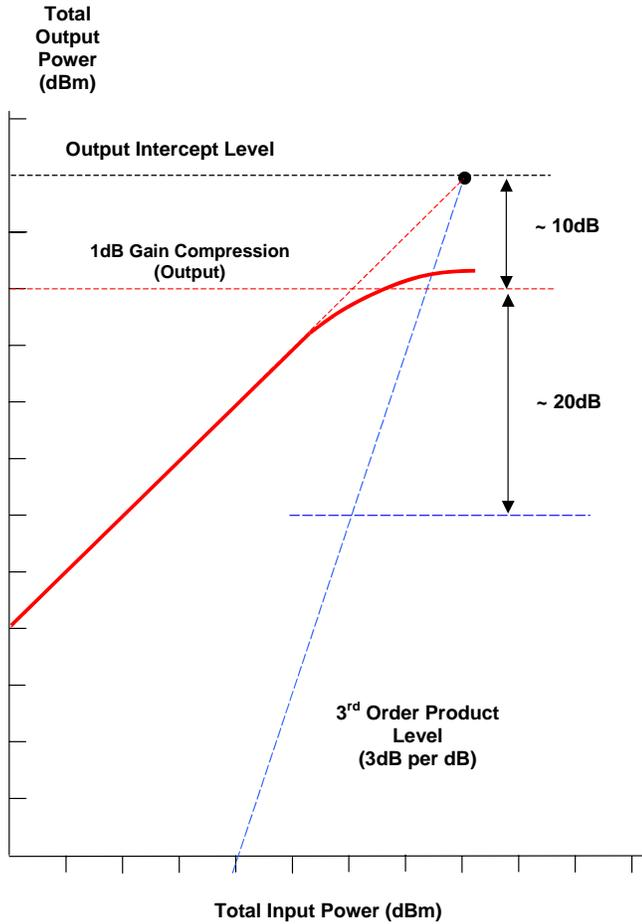
Figure 19 Plots of gain compression (red curve) and 3<sup>rd</sup> order intermodulation level (blue line) for a typical amplifier.
