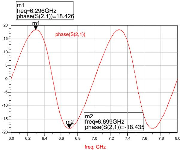
**Figure 6** Resulting phase vs frequency plot from the ADS S-parameter simulation shown in Figure 4, showing the predicted ~35 degree peak-to-peak phase ripple response due to the leaked back signal.
