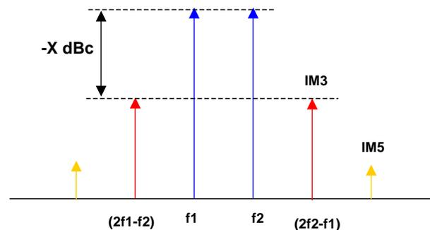
**Figure 18** Resulting carrier spectrum when two equal signals cause non-linearity in an active device.  $-X$  is the third order modulation product relative to the carrier in dBc.
