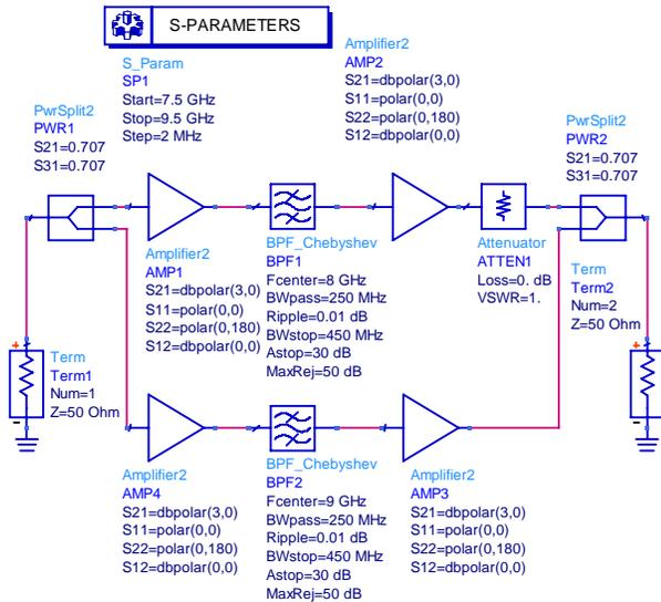
**Figure 14** ADS schematic to verify the multi-path hand calculations performed in the example. The filters have
