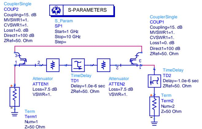
**Figure 8** ADS schematic to simulate the effects of feedforward radiation in attenuator blocks.
