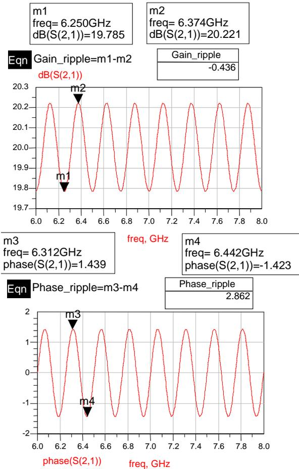
Figure 11 Resulting gain & phase ripple plots from the ADS simulation shown in Figure 10. The plots show agreement with the hand calculations presented in the example.
