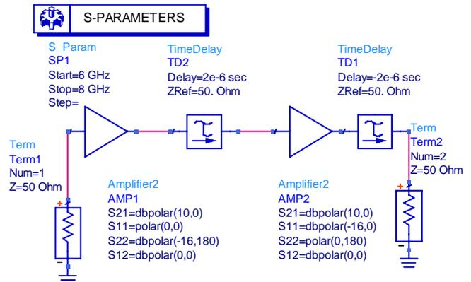
**Figure 10** S-Parameter ADS schematic to simulate effect of finite return losses. The first amplifier has been set up to have an output return loss of  $-16\text{dB}$ , with the second amplifier input return loss also set to  $-16\text{dB}$ . The delay of  $2\mu\text{s}$  is inserted to represent coaxial cables, micro-strip etc joining the two amplifiers. The second delay of  $-2\mu\text{s}$  takes out the electrical delay to leave the phase pk-pk response after simulation.
