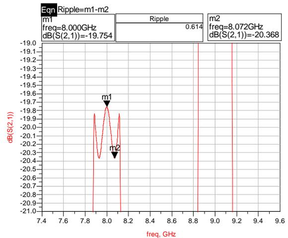
**Figure 16** Simulation result of the multi-path ADS schematic of Figure 14, with attenuator ATTEN1 set to 20dB in the wanted signal path. The plot verifies that the attenuator will degrade the gain ripple to ~0.55pk-pk.
