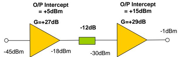
$$IM3 = -[5 - (-18)] \times 2 = -46 \text{dBc} \quad IM3 = -[15 - (-1)] \times 2 = -32 \text{dBc}$$
