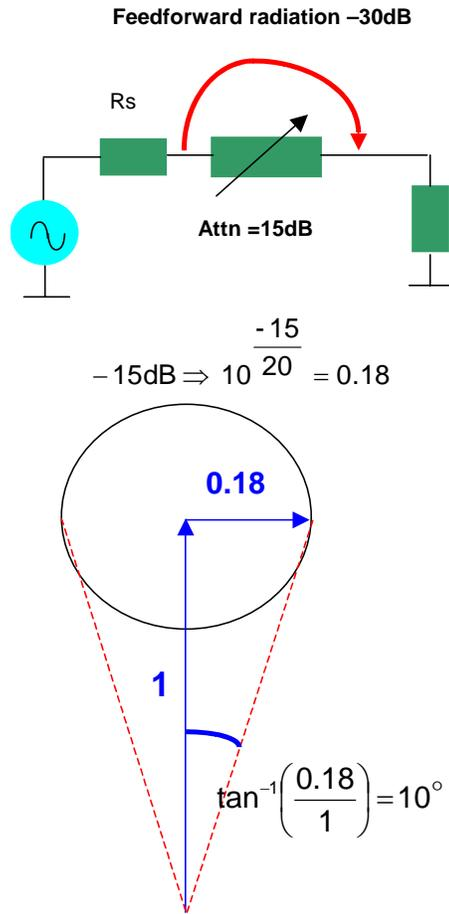
**Figure 7** Resulting phasor from feedforward radiation across the attenuator that will increase the gain/phase ripple.
