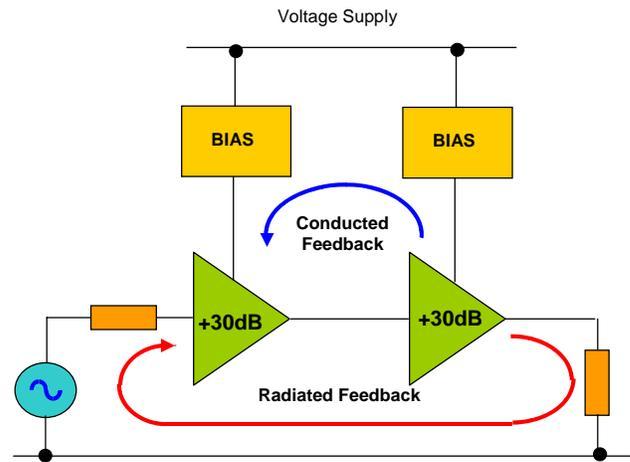
**Figure 2** Feedback paths that can degrade the gain ripple of a system.
