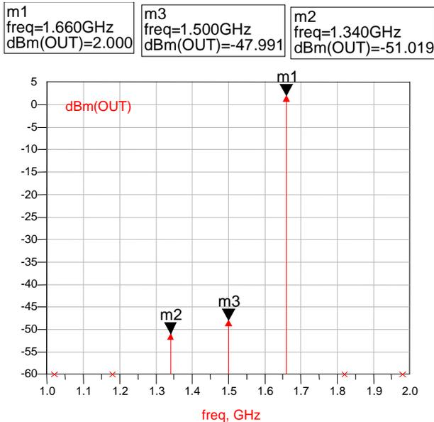
Figure 29 RF spectrum (dBm) of the simulation of Figure 27, with the LO rejection filter fitted and designed to have a stop-band rejection of 53dB, resulting in a S/LO ratio of 50dB, as per the example.
