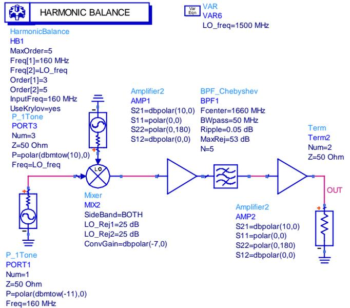
**Figure 27 Harmonic balance simulator to examine the LO leakage from a typical mixer. The RF and LO frequencies have to be specified in the harmonic balance simulator. The mixer is set to up-convert AND down-convert – Side Band BOTH, with a LO\_Rej2 (LO to Output Port) rejection of 25dB. Two simulations have been performed one without the filter to show the level of LO breakthrough and the second simulation with a filter added to give 50dB LO rejection.**
