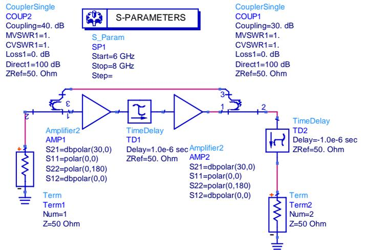
**Figure 4** ADS S-parameter schematic of the example amplifier chain shown in **Figure 2**. The signal is fed back from the output of the second amplifier, to the first amplifier input using two couplers of total coupling factor of 70dB. The electrical delay is to give the circuit some frequency dependence and is arbitrarily set at 1uS.
