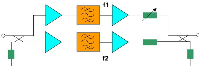
Figure 12 Schematic to illustrate the multi-path effect.
