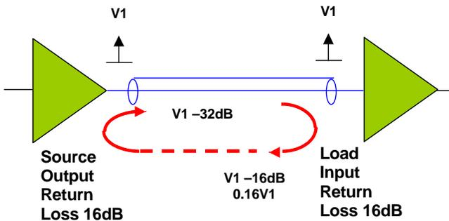
**Figure 9** Example circuit to show the effects of finite return losses on the gain uncertainty or gain/phase ripple.
