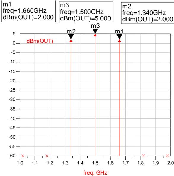
Figure 28 RF spectrum (dBm) of the simulation of Figure 27, with the LO rejection filter omitted, resulting in a S/LO ratio (Marker 3/Marker 1) of only 3dB, as per the example
