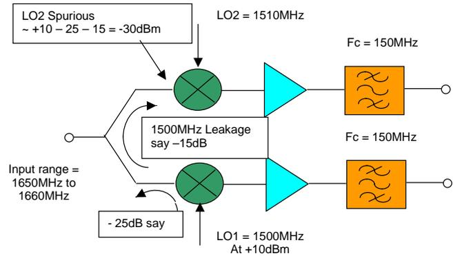
Figure 30 Multiplexed RF channels showing how the LO1 local oscillator can leak through to mixer 2 – at around -30dBm. This can then mix with the input signal at 1650MHz to give in-band spurious.
