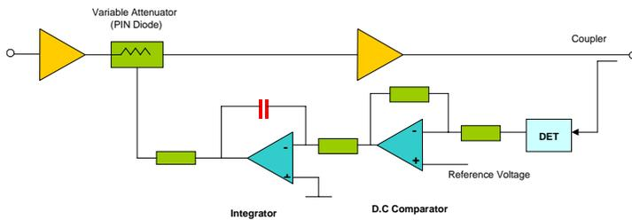
**Figure 21 Typical ALC arrangement**
